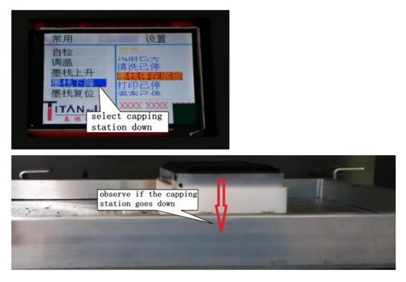
7.2. Select Capping station up to observe if capping station up, up to the top, the display screen shows the capping station stops at the top.
