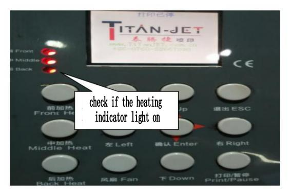
9. Press the Fan button on the keyboard (or go to Common menu - select the Fan), use hand to feel if fan is working properly, while observe if the LED lights are illuminated on the cover.
